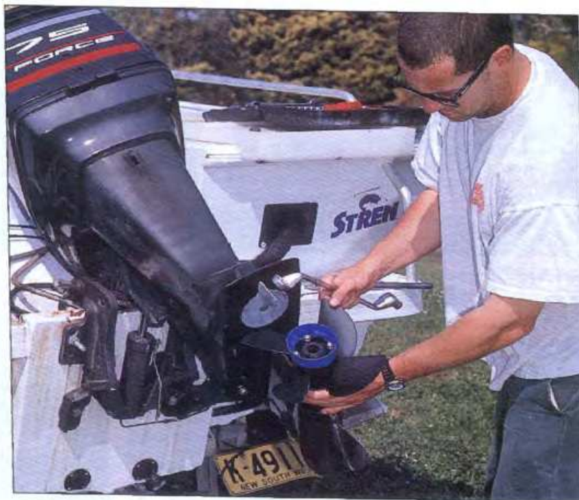
Fitting a ProPulse prop. Adjusting pitch, or replacing a blade is relatively easy although some may find it a tad 'fiddly'.
