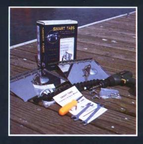
The Smart Tab system comes with all of the parts needed for installation. Here, the stainless steel tab plates, hinges and plate brackets have been pre-assembled according to the owner's manual, and optional zinc anodes have been added for saltwater use. Tools required include an electric drill, <sup>3</sup>/<sub>16</sub>-inch bit, countersink, Phillips screwdriver, two <sup>1</sup>/<sub>2</sub>-inch box-end wrenches, masking tape and marine sealant.
