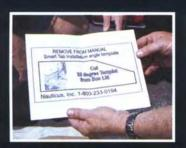
■ STEP 7: To set the angle of the tab, use the template in the owner's manual to create a cardboard jig, reflecting a 25-degree down angle.
