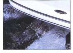
■ The stainless steel Smart Tabs are mounted much like hydraulic trim tabs, but the actuators are selfadjusting gas-spring struts that provide down force. Water rushing across the faces of the tabs creates lift.
