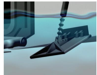
Trim tabs for small boats are also available, and highly effective for performance enhancement. These self-adjusting trim tabs work independently and require no operator interface. Automatic trim tabs are available from Nauticus with nitrogen gas-filled actuators. Nauticus trim tabs (SMART TABS®) are available in seven different models
